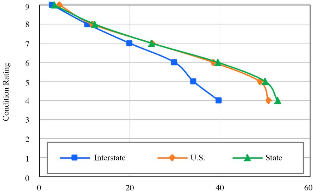
Figure 9. Deterioration model (A) Interstate highway, (B) U.S. highway, (C) State highway.
